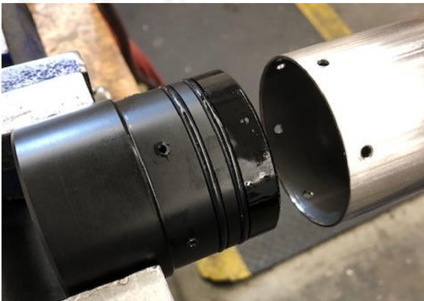
Photo 2 – Bottom End Cap Removal
