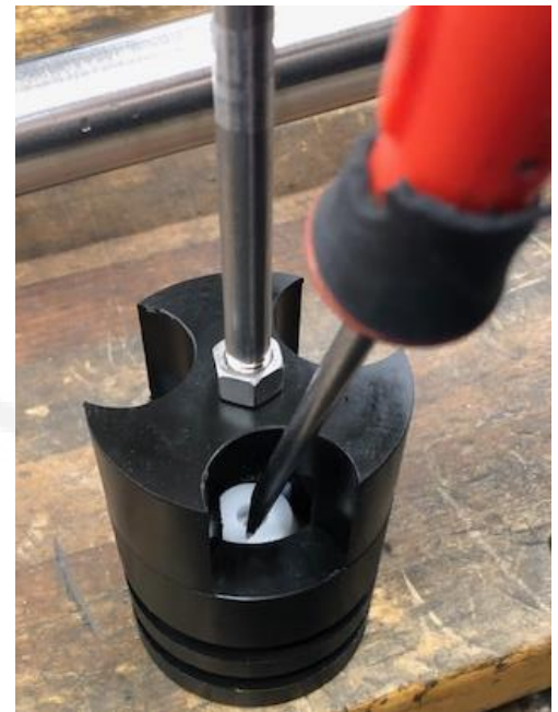
Photo 8.2 –Piston Check Valve Removal
