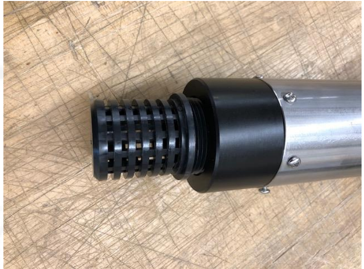
Photo 1 – Bottom End Cap with Filter
