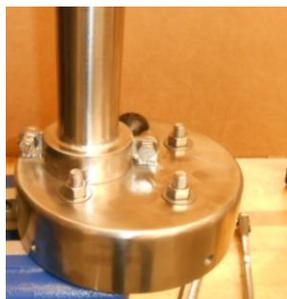
**STEP #11** – Remove the two bolts and the pump head exposing the lift rod and quick disconnect adapter and sleeve. Set off to the side. Install the well adapter onto the last piece of 1 ¼” pvc.
