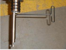
**STEP #15** - One person can steady the pump head while the second person can loosen the set screw on the quick disconnect sleeve using the 1/8" Allen Head Looped Wrench that is provided in the kit. Now slide the sleeve down over the two adapters until it stops. Retighten the set screw. Now lower the entire pump head into the well adapter quick disconnect sleeve engaging the o-rings. Line up the
