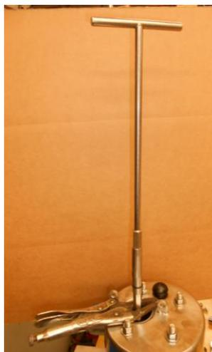
**STEP #14** – Thread the extra quick disconnect rod adapter onto the rod retrieval tool. Use this to connect to the adapter on the last piece of pipe and rod. Lift up through the well adapter and hold with vice grips.
