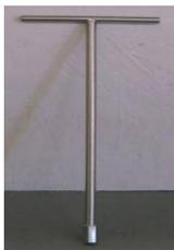
**STEP #13** – Attach the rod retrieval tool to the last section of rod and pull all the way up. Attach vice grips to hold the rod up from the pipe.
