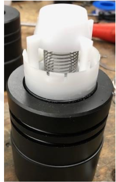
Photo 6 – Check Valve Orientation
