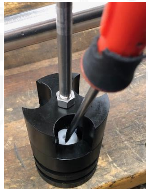
Photo 8.3 –Piston Check Valve Removal
