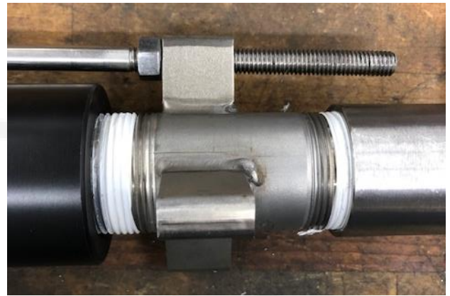
Photo 1 – Longer Threaded End of Tie Rod
