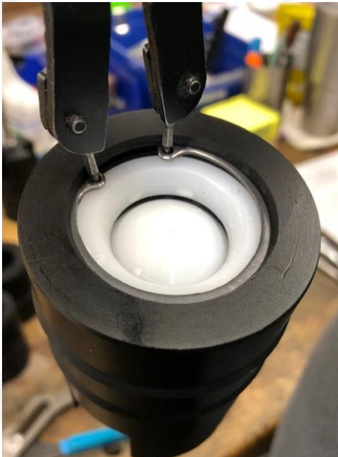
Photo 8.2 –Piston Snap Ring Removal
