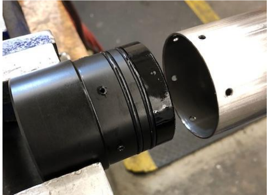
Photo 2 – Bottom End Cap Removal
