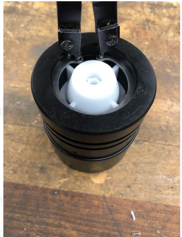
Photo 4 – Internal Snap Ring Removal
