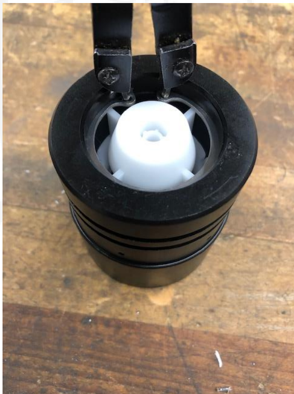
Photo 4 – Internal Snap Ring Removal
