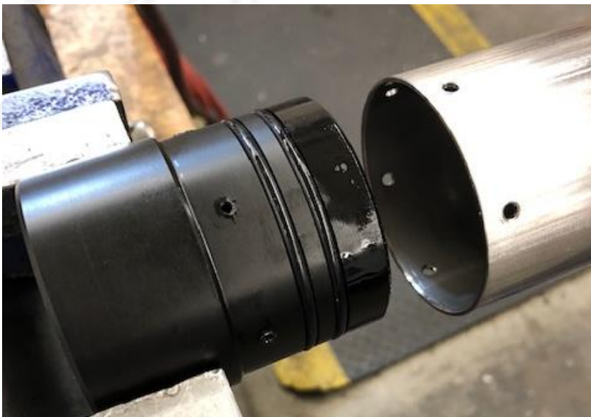
Photo 2 – Bottom End Cap Removal
