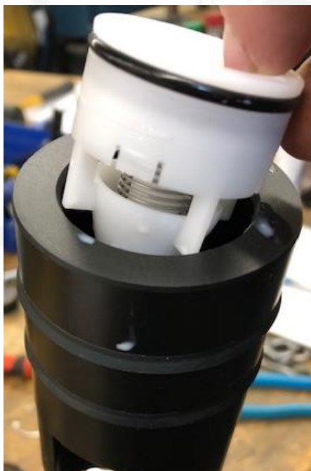
Photo 9 – Piston Check Valve Orientation
