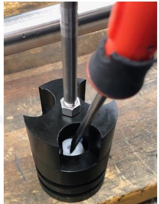
Photo 8.2 –Piston Check Valve Removal
