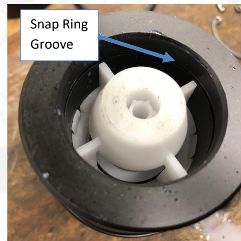
Photo 7 – Check Valve Placement
