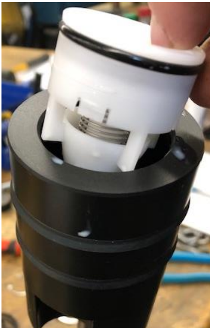
Photo 9 – Piston Check Valve Orientation
