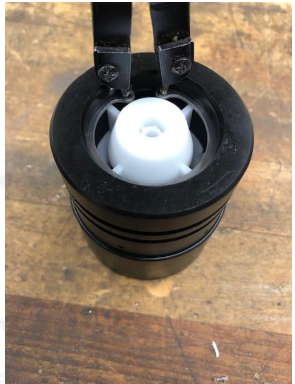
Photo 4 – Internal Snap Ring Removal
