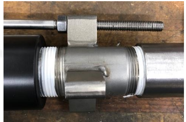
Photo 1 – Longer Threaded End of Tie Rod
