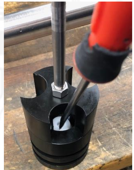
Photo 8.3 –Piston Check Valve Removal
