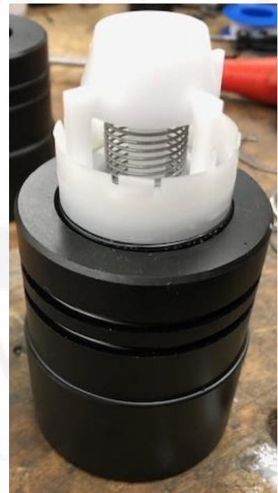
Photo 6 – Check Valve Orientation
