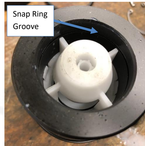
Photo 7 – Check Valve Placement
